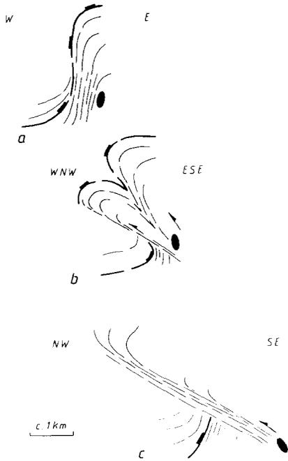
Fig. 12. Sketch sections illustrating the variation in styles of compressional structures along the western margin of the Nanga Parbat syntaxis. (a) Sassi, (b) Ramghat, (c) Raikhot. The brick-ornamented line represents the MMT.
