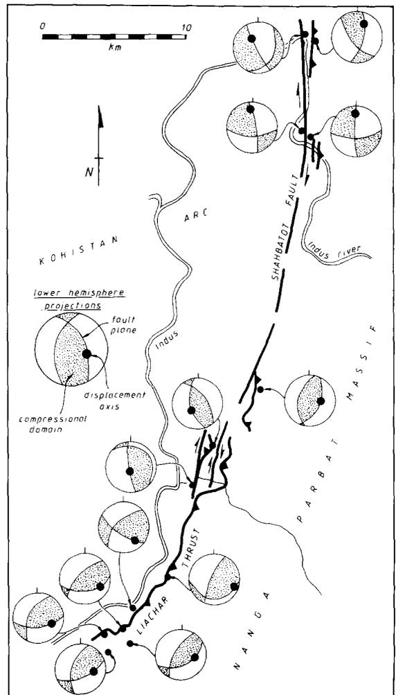
Fig. 13. Palaeofault plane solution map of western margin of the Nanga Parbat massif, based on structural kinematic indicators in fault zones recorded by the authors. The area of the map is as for Fig. 3.
