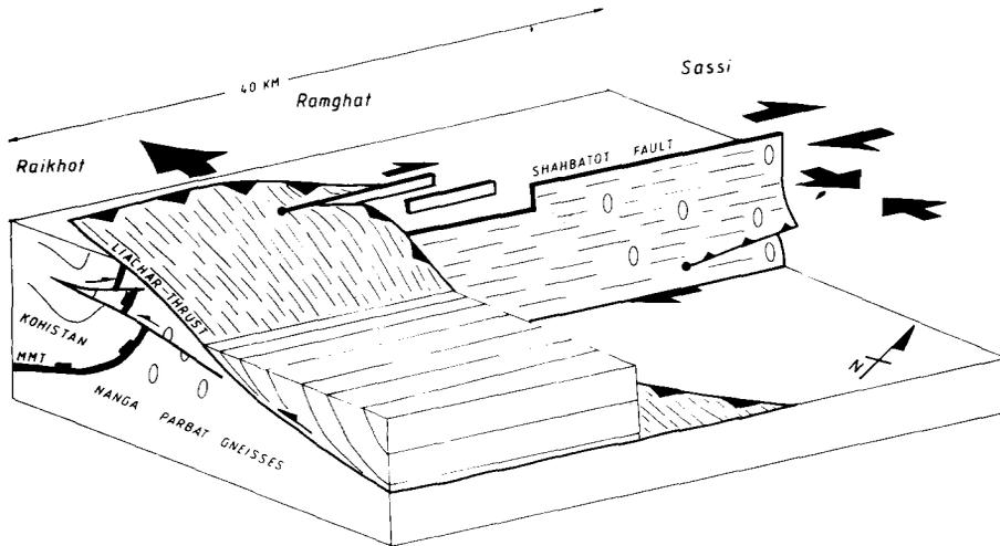
Fig. 14. Stylised block diagram showing the interpreted relationship between thrust and strike-slip fault zones along the western margin of the Nanga Parbat syntaxis. High-level cataclastic fault zones which form the pattern apparently migrated southwards with time so that strike-slip overprints thrusting.
