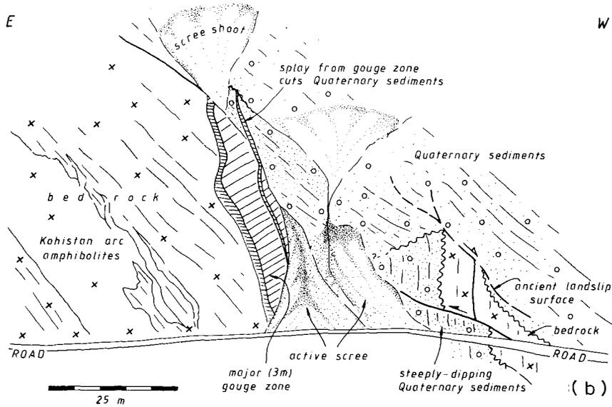
Fig. 9. (a) View of the relationships between bedrock (Kohistan complex gneisses and metagabbro) and Quaternary Indus valley sediments in the lower Astor Valley, near its confluence with the Indus (*f* in Fig. 3). The major gouge zone is arrowed. (b) Interpretation of the above, based on detailed field observations.
