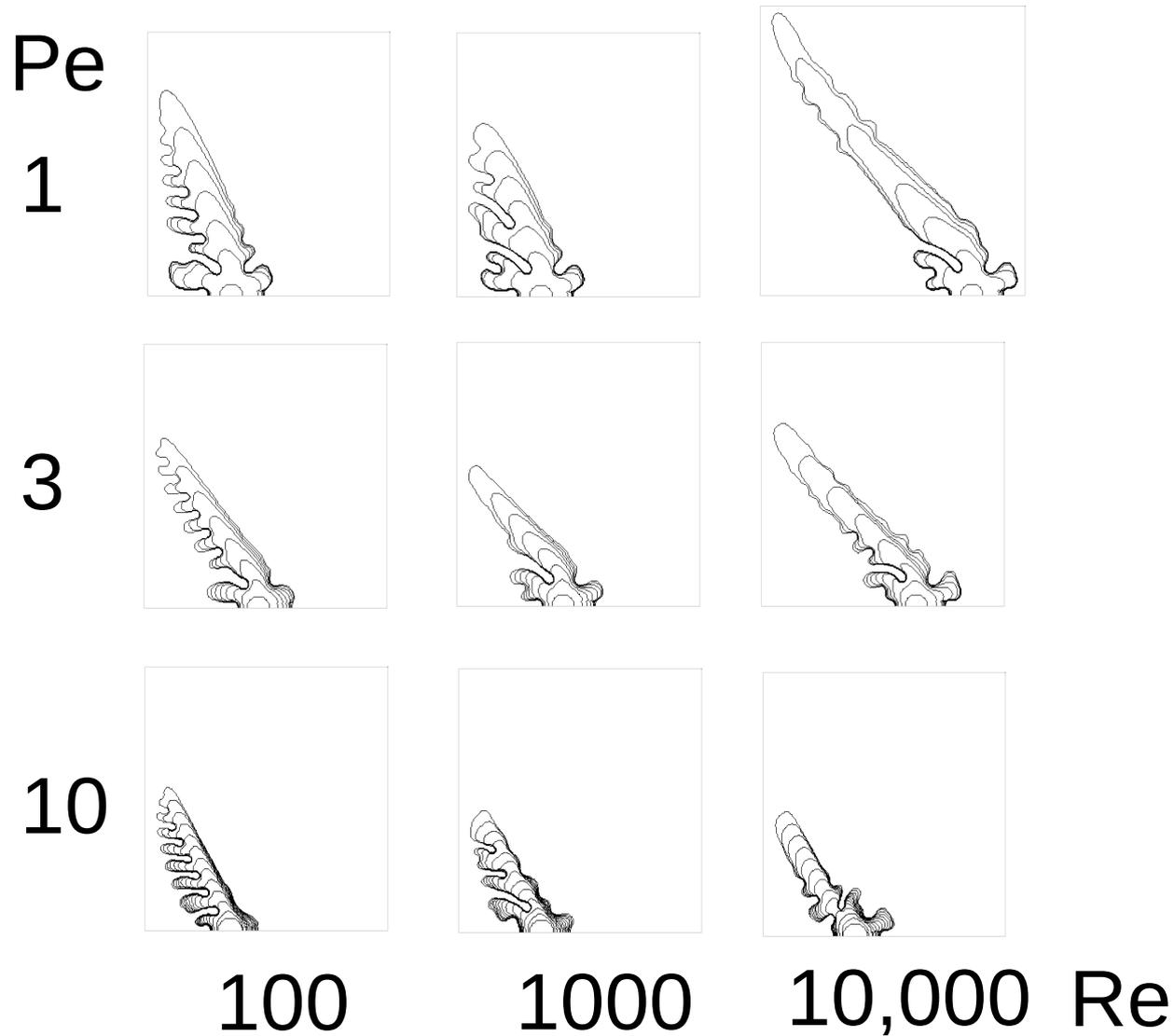
Difference in morphology for various changes in physical parameters (orientation, shape, growth rate)
