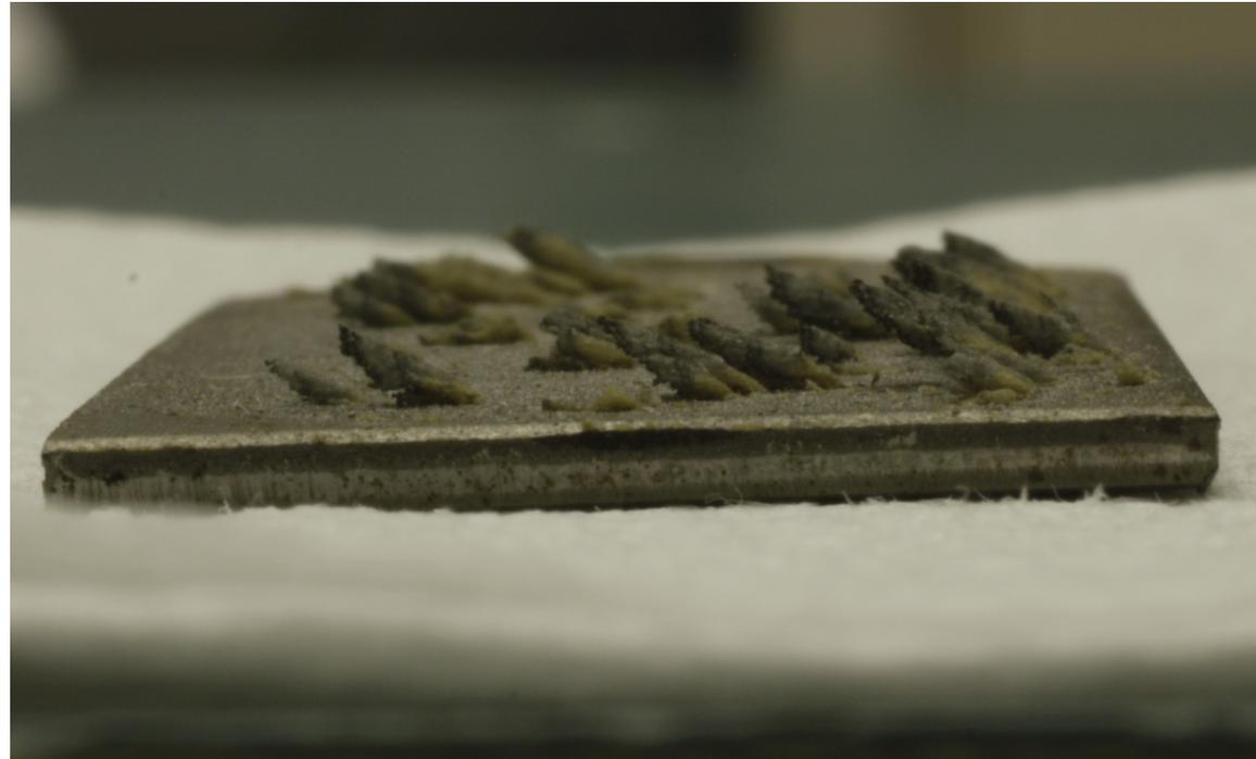
Samples of precipitation from hydro-thermal pipelines in Iceland
