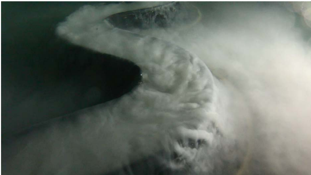
Figure 1. View of flow through a laboratory underwater river. Flow is towards the viewer, and can be seen to be spilling over the sides of the channel. The channel is approximately 20 cm wide.
