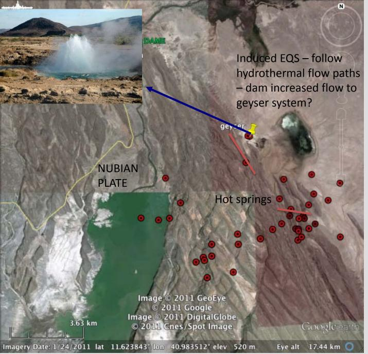
Red dots are EQs located by AAU-NSF array in 2009 after dam filling. Most occurred as swarms in February-July, 2009.
