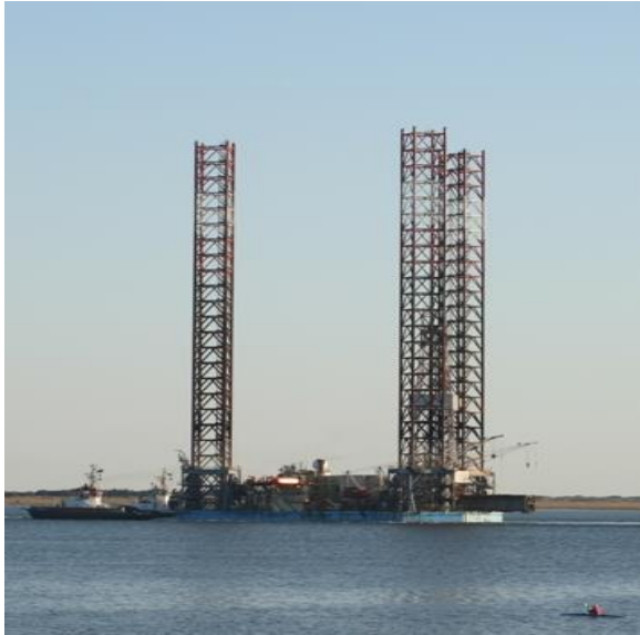
Jack-up rig during towage, with legs elevated
