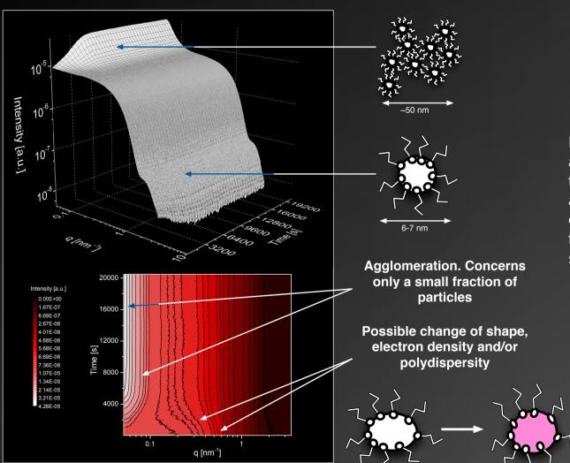
Precipitation of calcium carbonate amorphous nanoparticles in microemulsions followed by in situ and time-resolved small angle X-ray scattering. Two scattering contributions are clearly visible: (1) scattering from individual micelles at high-q and (2) scattering from agglomerates at low-q.
