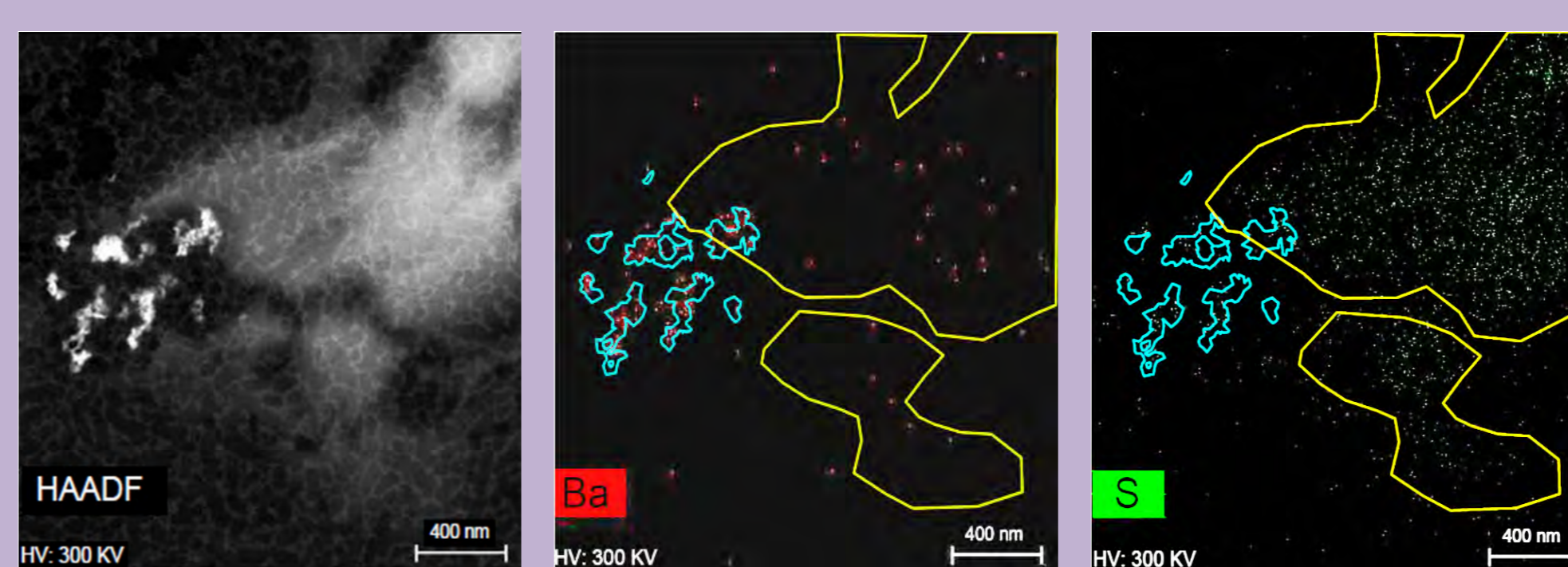
Fig. 3. The first image is high angle annular dark field image (HAADF) taken in STEM mode using FEI-TITAN. The line in blue delimited the aggregates of barium sulphate nanorod particles and the yellow line is around the "ghost" area. EDX mapping carried out in this area. Ba and S are mainly concentrated in the "ghost" area.
