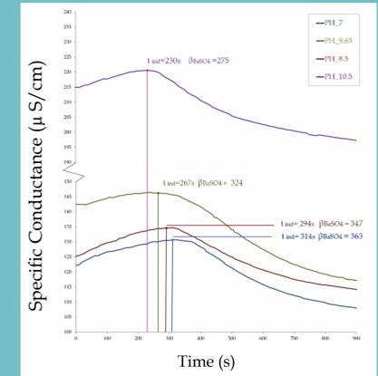
Fig. 4. Specific conductance ( $\mu\text{S/cm}$ ) as function of time for different pH values.
