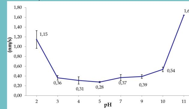
Fig 1. Growth rate in the [001] direction as function of pH.
