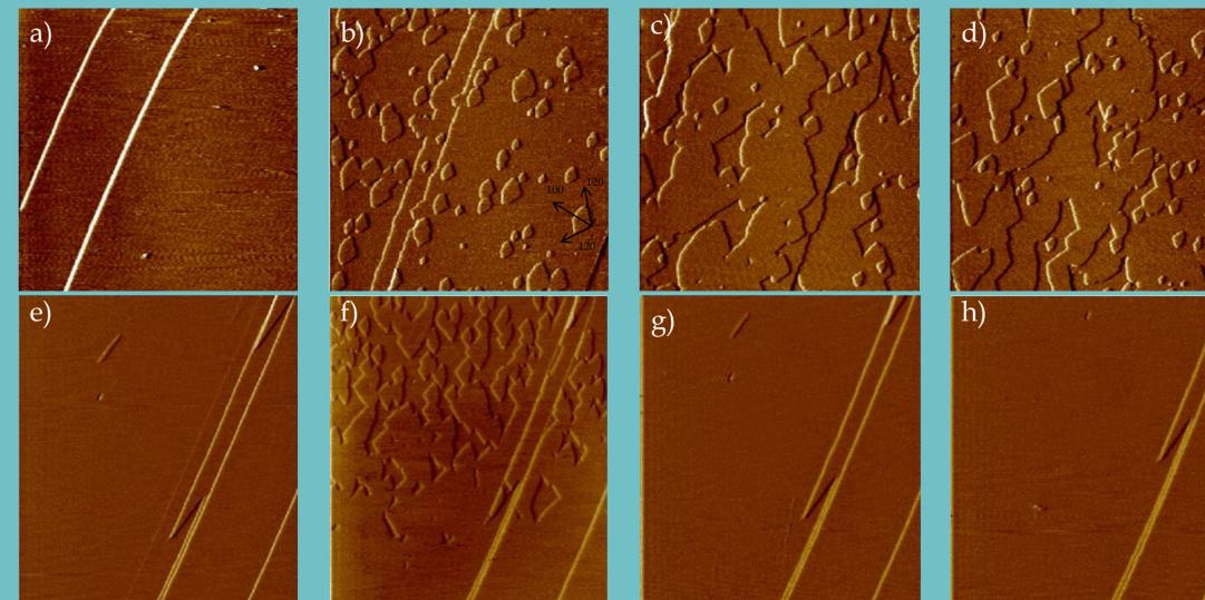
Fig 2. AFM deflection images of growth of (001)  $\text{BaSO}_4$  surface at SI= 0.92 and (a-d) pH = 7 and (e-h) pH=12. Size of the image is 5  $\mu\text{m}$ .
