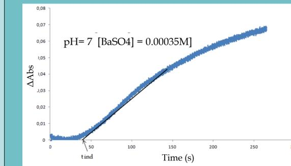
Fig. 3. Typical evolution of turbidimetry (expressed as absorbance) during precipitation experiments.
