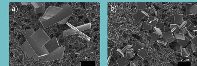
Fig. 5. FESEM images of  $\text{BaSO}_4$  precipitates formed at (a) pH=7 and (b) pH=11 and SI=2.24.
