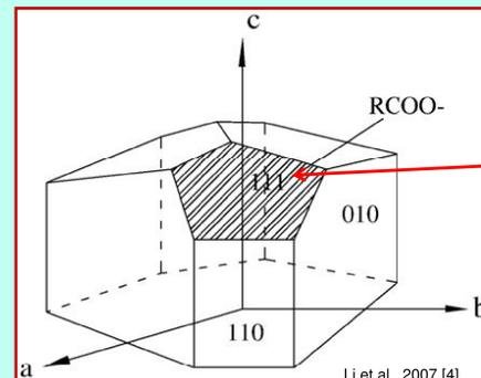
Fig. 8. Schematic of likely sorption of carboxylic group on gypsum growth site
