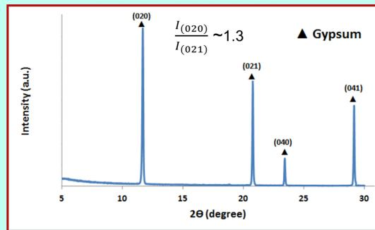
Fig. 12. XRD pattern of precipitates from system with 20ppm citric acid and pH 7 after 200min
