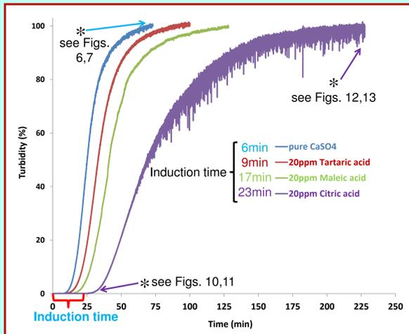
Fig. 3. The effect of various carboxylic acids on the precipitation of calcium sulfates.
