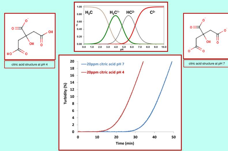
Fig. 5. How the pH dependent citric acid speciation is affecting the inhibition performance in the calcium sulfate system
