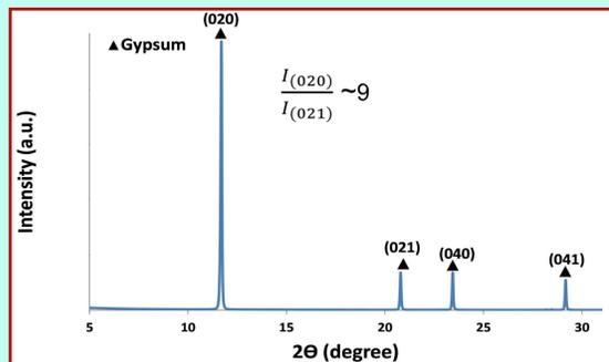
Fig. 7. XRD pattern of precipitates from the additive free system after 75min
