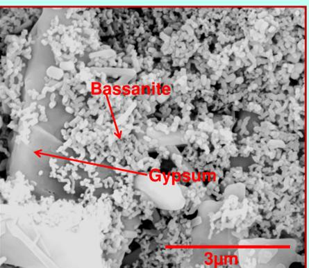
Fig. 10. SEM image of gypsum and bassanite formed at pH 7 with 20ppm citric acid after 28min
