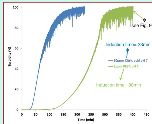
Fig. 4. Comparison between the effect of 20 ppm citric acid and 5 ppm PESA on calcium sulfate precipitation.
