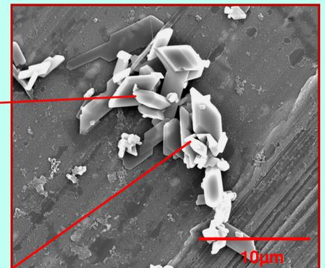
Fig. 9. Photomicrograph of gypsum crystals in the system with 5ppm PESA and pH 7 after 400min
