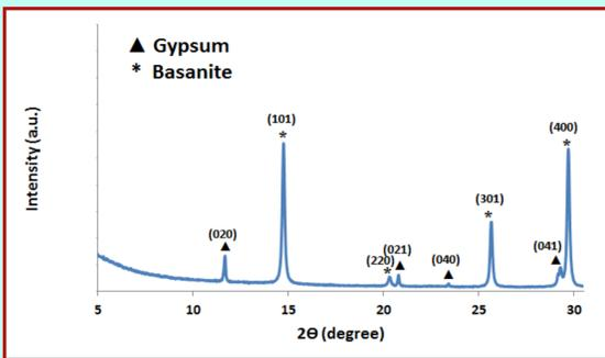
Fig. 11. XRD pattern of precipitates from system with 20ppm citric acid and pH 7 after 28min
