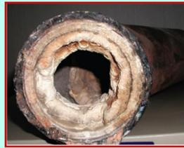
Fig. 1. Mineral scaling reduces fluid flow
