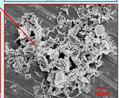
Fig. 13. Photomicrograph of gypsum plates in system with 20ppm citric acid and pH 7 after 200min
