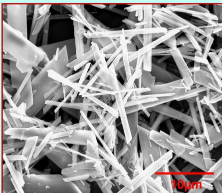
Fig. 6. Photomicrograph of gypsum needles formed without additives
