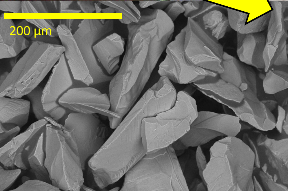
SEM images of unreacted forsterite loaded to flow through reactor experiment.
