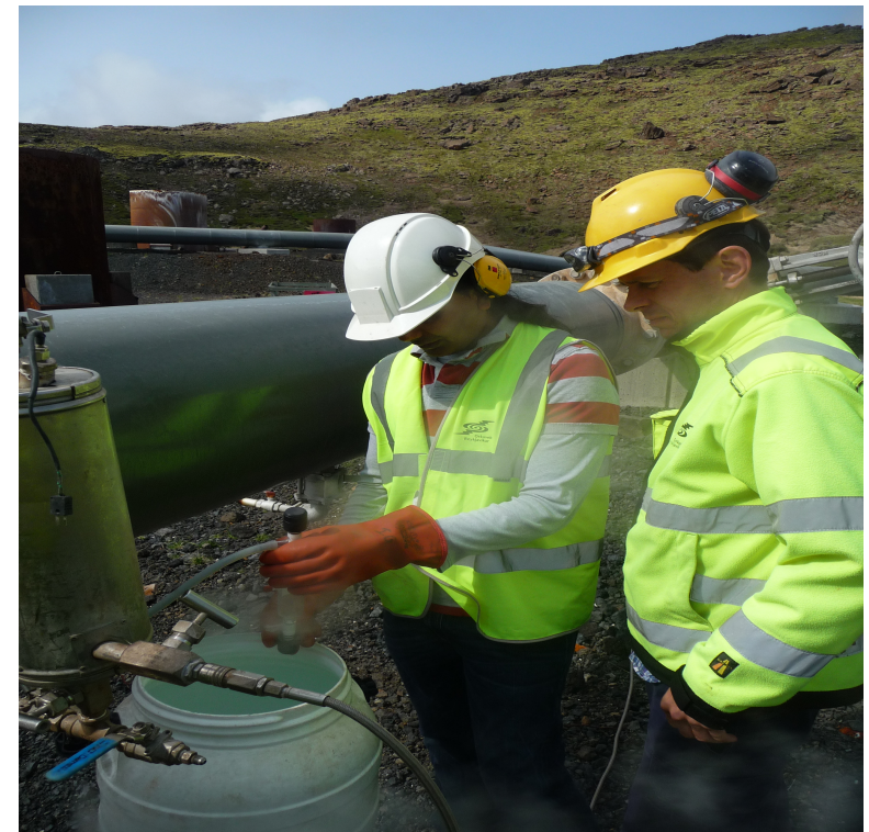
Fig 2. Sampling at high temperature geothermal well
