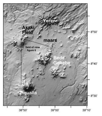
**Fig. 4.** Shaded DEM (SRTM – NASA/JPL) of the Debre Zeyit region of the SDFZ. Large silicic volcances are labeled (Yerer, Ziqualla, and Bede Gebebe). The Pliocene Akaki cinder cone field is shown adjacent to the SDFZ. The SDFZ terminates ~9°N against a protrusion of the Ethiopian Plateau (Boru-Toru Structural High; Bonini et al., 2005). Note the abundance of cinder cones and maars along the alignment of the SDFZ which cut the earlier Bede Gebebe edifice.
